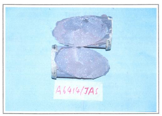
Photograph 3: Shows bond failure of Sikadur 731 Epoxy Resin Adhesive between the two half-cylinders at 14 days of age.
