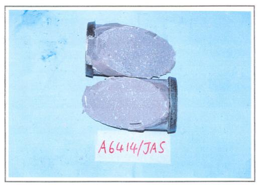
Photograph 2 : Shows bond failure of Sikadur 731 Epoxy Resin Adhesive between the two half-cylinders at 2 days of age.
